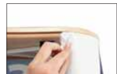
Fitting graphics into SEG channel
